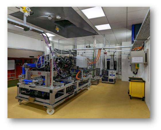
The Company assembled and set-up its first **Fuel Cell Power Module (FCPM)** for demonstration at its Research and Development facility at Bangalore.
