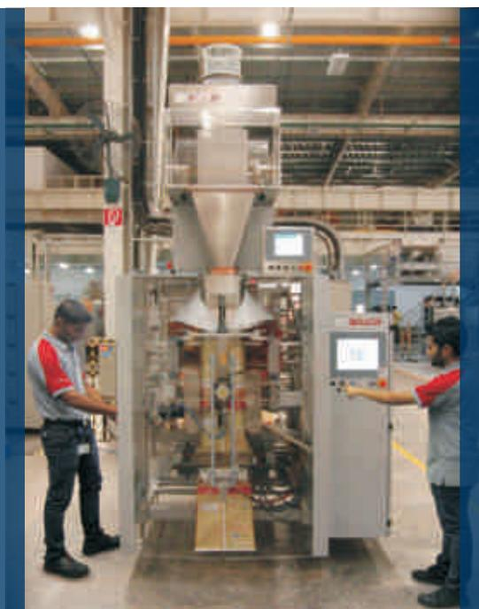
Indigenously developed, the vertical-form-fill-seal packaging machine SVI 4000 is used for packing products like rice, grains, pulses, seeds and non-food products.
